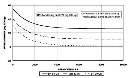
It is recommended to use in the first place BN 50 - 55 lubricants when operating on heavy fuel. This recommendation is valid especially for engines having wet lubricating oil sump and using heavy fuel with sulphur content above 2,0 % mass. BN 40 lubricants can be used when operating on heavy fuel as well if experience shows that the lubricating oil BN equilibrium remains at an acceptable level.
